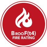
Both products achieve a BROOF(t4) designation in accordance with EN 13501-5 & equivalent BS476-3 fire rating for full UK & EU compliance. These results mean no restrictions to boundary construction.
